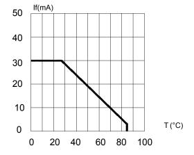
Fig. 5 Forward Current vs. Temperature
