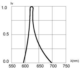
Fig. 1 Relative Luminous Intensity vs. Wavelength @ 20mA
