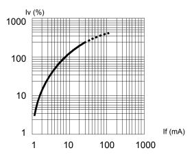
Fig. 4 Relative Luminous Intensity (%) vs. Forward Current
