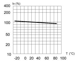
Fig. 6 Relative Intensity (%) vs. Temperature @ 20 mA
