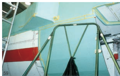
59 Abrasion-resistant rubber backing and acrylic adhesive of 3M™ Impact Stripping Tapes protect surfaces during plastic media blasting.
