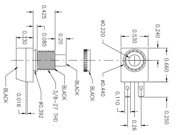
JUDCO INVENTORY NO. 40-4524-00 SWITCH TYPE: PUSH ON-PUSH OFF, SPST UL ELECTRICAL RATING: 125 VAC, 6A UL TEMPERATURE RATING: 65°C NUT PACKED SEPARATELY
