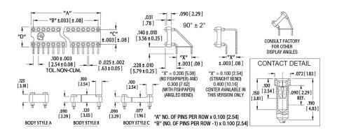
ALL DIMENSIONS: INCHES [MILLIMETERS] ALL TOLERANCES: ±0.005 [0.13] UNLESS OTHERWISE SPECIFIED FOR VERTICAL MOUNTING, SEE DATA SHEET 13002 **CONSULT FACTORY FOR OTHER SIZES AND CONFIGURATIONS**
