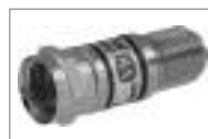
'F' Mini-Attenuator Pads Nickel Plated, Accuracy within 5%, Return Loss 20db, 22 AWG Center Pin, DC to 1 GHz Bandwidth, (M) to (F)
