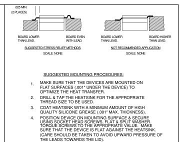
SOLDER LEADS IN PLACE USING APPROPROATE SOLDER WITH A CONTROLLED TEMPERATURE IRON.
