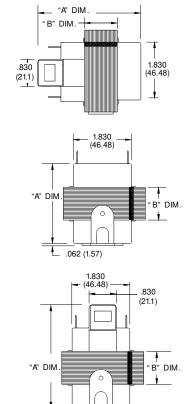
"A" and "B" Dimensions for 60VA & 75VA Models
