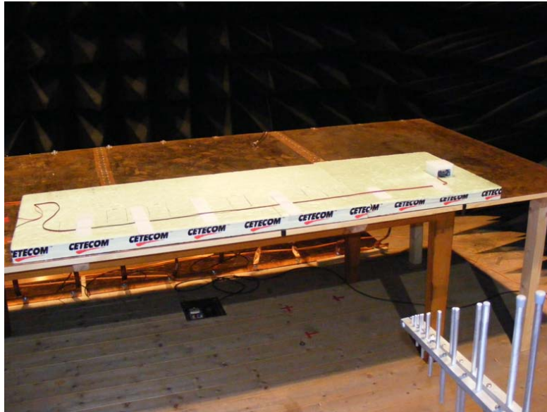
Photo 2: Emission Stripline 500 kHz - 1000 MHz
