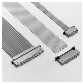
This extremely small 0.5mm (.020") pitch connector with a height of only 2.0mm (.079") above the PCB surface allows interconnection in extremely small spaces and is an example of JST's leading edge technology.
