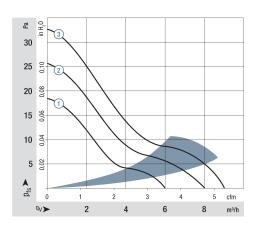
Air performance measured according to: ISO 5801. Installation category A, without contact protection. Noise: Total sound power level L<sub>W</sub>A ISO 103002 measured on a hemisphere with a radius of 2 m. Sound pressure level L<sub>P</sub>A measured at 1 m distance from fan axis.
