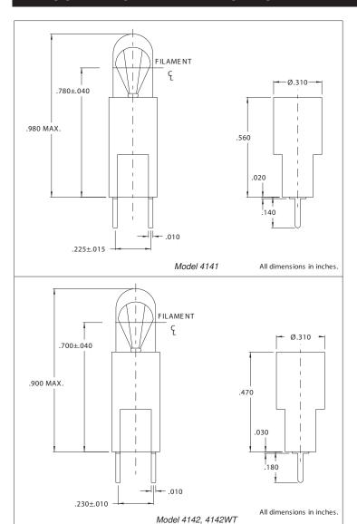
Mounting: Printed circuit Board
