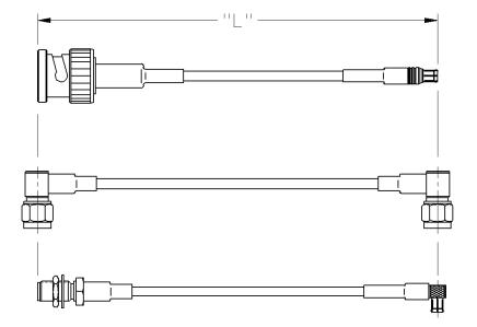
Johnson Components' cable length applies to the end of straight connectors. The length is applied to the vertical centroid of right angle connectors.
