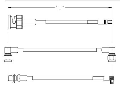
Johnson Components' cable length applies to the end of straight connectors. The length is applied to the vertical centroid of right angle connectors.
