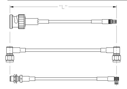
Johnson Components' cable length applies to the end of straight connectors. The length is applied to the vertical centroid of right angle connectors.
