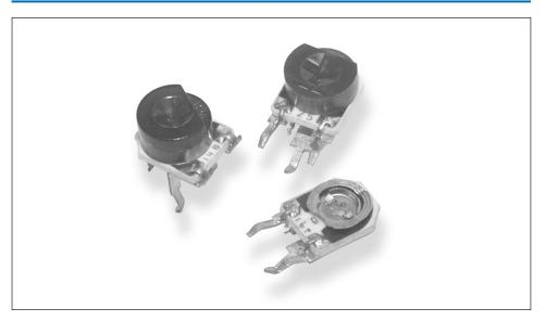
This tiny 6mm square cermet trimmer is offered with alternative adjustment covers for screwdriver and automatic setting and can be supplied in bulk or taped in ammo pack. The 416 can be adjusted from the top or side and is an inexpensive solution to high reliability potentiometer requirements. This series is used to replace some of the larger, expensive, sealed types in high volume circuits.
