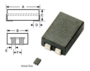
**Mechanical Configuration** Ferrite bead with plated copper wire. Provides a common path for the magnetic flux generated by the current to and from the load. The resulting effect is zero magnetics flux in the core.
