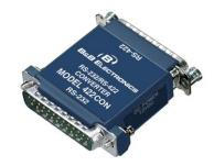
The RS-232 port uses a male DB25 type of connector with pins 2(TD input) and 3(RD output) supported. Protective ground (pin 1) and Signal Ground (pin 7) are also connected. The RS-422 port uses a female DB-25 type of connector with the Send Data outputs on pins 2 and 14, and the Receive Data inputs on pins 5 and 17. Protective Ground (pin 1) and Signal Ground (pin 7) are connected through to the RS-232 connector.
