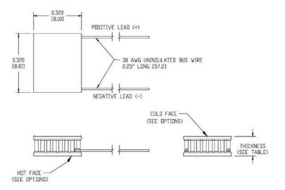
Ceramic Material: 96% Alumina Ceramics Solder Construction: 138°C BiSn
