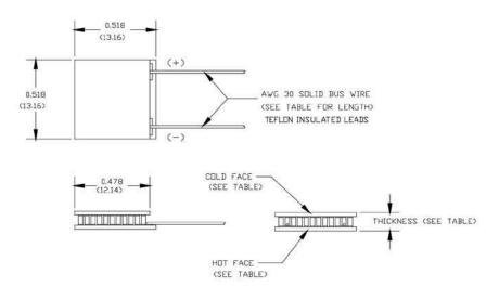
Ceramic Material: 96% Alumina Ceramics Solder Construction: 271°C, Proprietary
