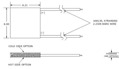
Ceramic Material: Alumina Nitride(AlN) Solder Construction: 232°C SbSn
