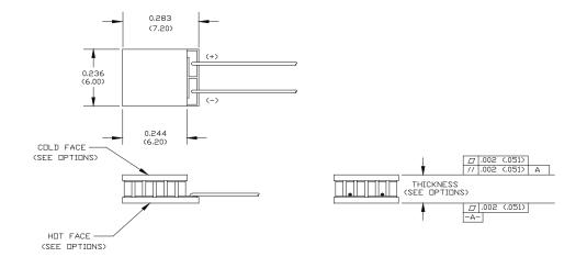
Solder Construction: 138°C, Bismuth Tin Tlam Substrates
