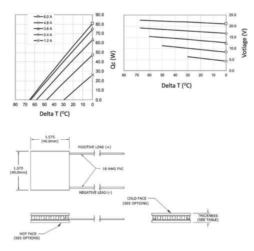
Ceramic Material: Alumina (Al<sub>2</sub>O<sub>3</sub>) Solder Construction: 138°C, Bismuth Tin (BiSn)
