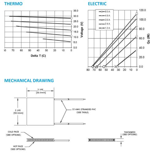
Ceramic material 96% Alumina ceramics Solder construction: 138°C BiSn
