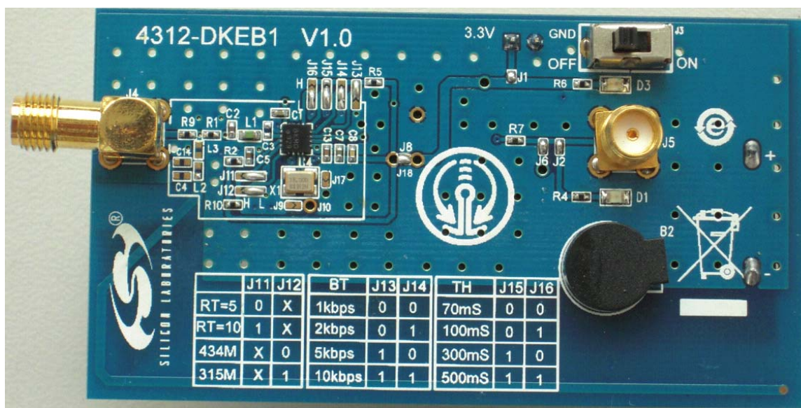
Figure 1. Si4312 DEMO Board Top Side
