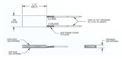
Ceramic Material: Alumina (AI<sub>2</sub>O<sub>3</sub>)
