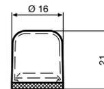
Protective transparent cover, degree of protection IP54
