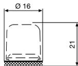
Protective transparent cover, degree of protection IP54
