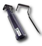
Professional stripping tool for cables of all insulations types. Positive locking positions for circular, lengthways and spiral strips. Interchangeable cable retention hooks give cable stripping capacity of up to 40mm/1.57 inch diameter. Replacement cutting blades can be stored within the tool.
