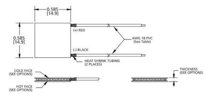
Ceramic Material: Alumina (Al<sub>2</sub>O<sub>3</sub>)
