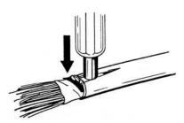
5.03 Place connector top over stud and tighten firmly with securing nut. Torque nut to 40-50 in-lbs (5.2±0.6 kgm) with company approved tool.
