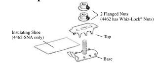
Note: Visually inspect all components. If any component is missing or appears damaged, do not install and call 3M customer service at 1-800-426-8688 for a replacement product. Note: On cables less than 3/4" (19 mm) in diameter, cut a 1 1/2" (38 mm) slit in the sheath opposite connector location. Then complete procedure.
