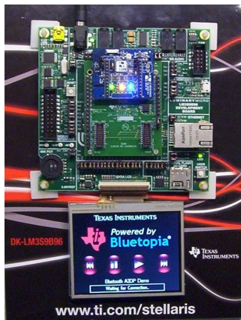
Figure 9 TiWi-uB2 EM Board with Stellaris DK-LM3S9B96
