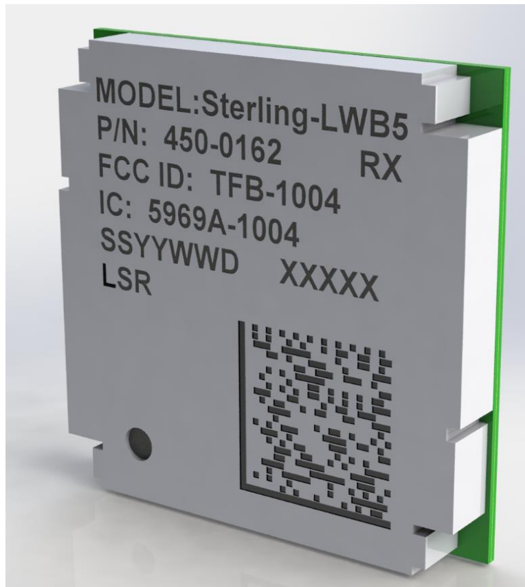
Figure 1 Sterling-LWB5 Base SIP Module (450-0162)
