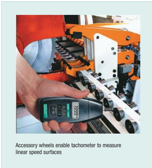
Accessory wheels enable tachometer to measure linear speed surfaces
