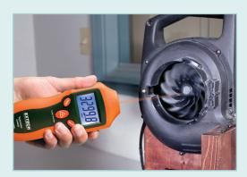
Non-contact fan blade RPM or REV testing
