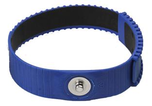
The Wristband 4600 Series consists of an insulative exterior with conductive interior and metal male snap available in 4mm. Made of thermoplastic material, the Wristband 4600 Series is lightweight, low profile and safely makes contact with human skin, assuring employee acceptance while helping to ensure ease of use. The "zipper" style latching mechanism easily adjusts to most wrist sizes.
