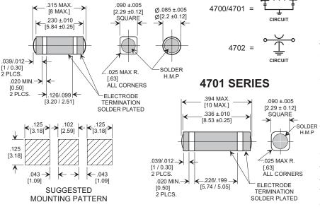
Dielectric Withstanding - 300VDC Direct Current Rating - 10 ADC Inductance Value - 100nH Minimum
