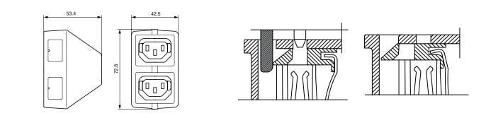
Shutter operation: shutters opened by plug insertion
