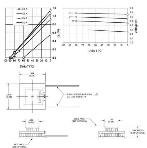
Ceramic Material: Alumina (AI<sub>2</sub>O<sub>3</sub>)
