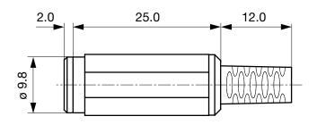
Cable diameter max. 4.0 mm
