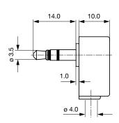
Cable diameter max. 4.0 mm
