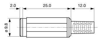
Cable diameter max. 4.0 mm
