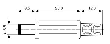
Cable diameter max. 4.0 mm
