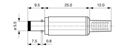
Cable diameter max. 4.0 mm
