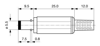
Cable diameter max. 4.0 mm
