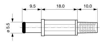
Cable diameter max. 4.0 mm
