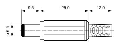
Cable diameter max. 4.0 mm
