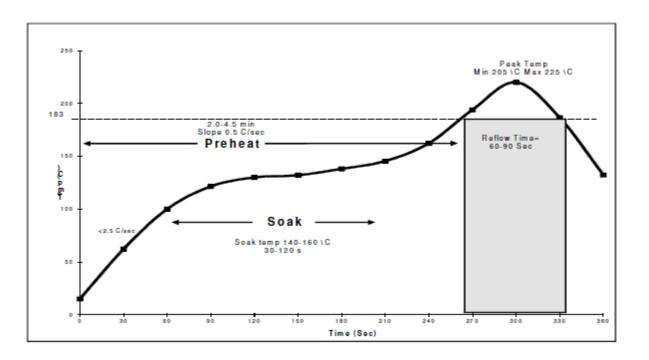
**Preheat Zone**—The preheat zone, which is also referred to as the ramp zone, is used to elevate the temperature of the PCB to the desired soak temperature. In the preheat zone, the rate of temperature rise should not exceed 2.5 °C/s to avoid thermal chock stresses. The oven preheat zone normally occupies 25–33% of the heated tunnel length.
