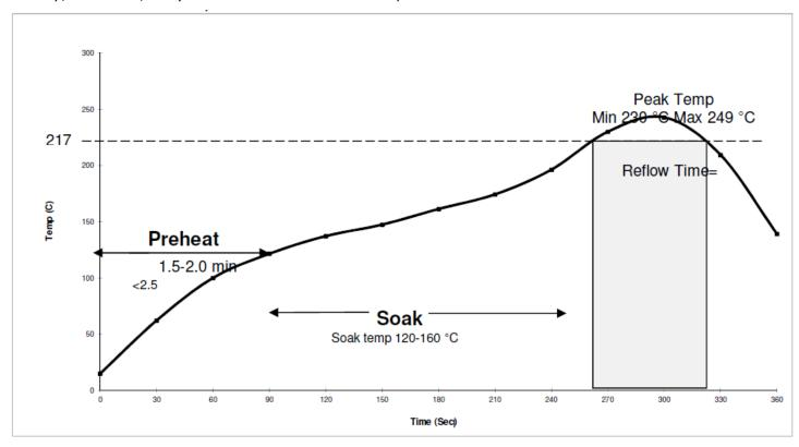
**The Preheat Zone**, which is also referred to as the ramp zone, is used to elevate the temperature of the PCB to the desired soak temperature. In the preheat zone, the rate of temperature rise should not exceed 2.5 °C/s to avoid thermal chock stresses. The oven preheat zone normally occupies 25–33% of the heated tunnel length.
