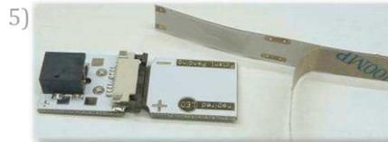
Now select the tiger paw that matches the polarity of the flexible LED strip end you would like to terminate. Peel back the adhesive liner on the LED strip about 1.5 inches. Please note that solder pads with a bump of solder on them cannot be terminated with this item.
