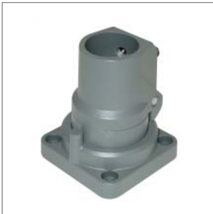
Foot stand, swivelling Cast aluminium with steel inner tube and flange mounting. Swivelling range 250° (cannot be limited or stopped) Order No. 49.49 68 00
