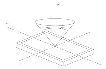
Inspection should be performed within angle  $\phi$  ( $\phi$  is usually 30°) from Z axis to each X and Y.
